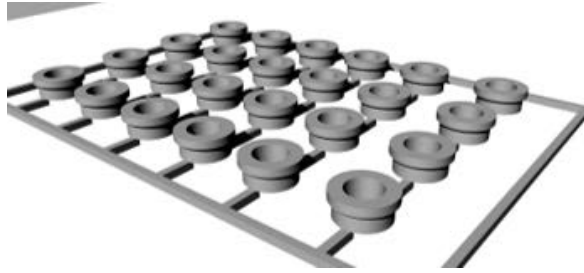
Supplementary Figure 1: Design for mesentery extraction scaffolds made using Rhino 5. Each cylinder has an external diameter of 0.7 cm
